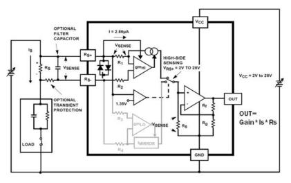
FIGURE 2. ISL28006 HIGHLY INTEGRATED AND ACCURATE CURRENT SENSE AMPLIFIER
