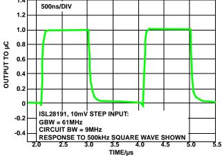
FIGURE 7. SIMULATED RESPONSE OF THE CIRCUIT IN FIGURE 5 TO A 10MV<sub>P-P</sub> SQUARE WAVE AT "Vc1". THE ISL28191 IS USED IN PLACE OF THE ISL28133
