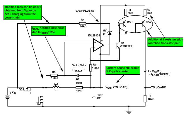
FIGURE 5. MODIFIED SENSE CONFIGURATION USING DCR SENSING IN A BUCK CONVERTER
