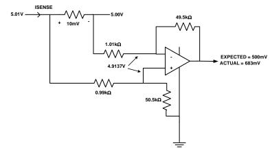
FIGURE 3. DIFFERENCE AMP CONFIGURATION WITH WORST CASED 1% TOLERANCED RESISTORS (1k $\Omega$  and 50k $\Omega$ )
